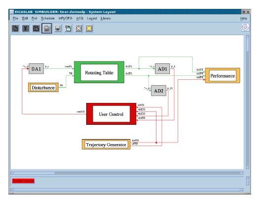
The Plant Area is used to program the model of the plant. Continuous, discrete or hybrid plants can be simulated.
