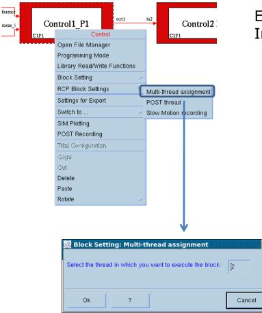
Every Control function and Processor Input/Output has to be associated to a thread.
